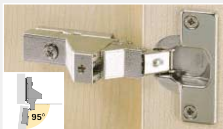
Intermat 9945 for door overlay adjustment 12 mm Opening angle 95° Pages 3.106 – 3.107
