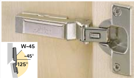
Intermat 9944 W -45 / 9944 W -45 FIX for negative cabinet angle -45° Opening angle 125° Pages 3.76 – 3.79
