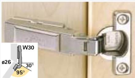
Intermat 9924 W30 for smaller doors / narrow frame doors Cabinet face angle 30° Opening angle 95° Pages 3.86 – 3.87
