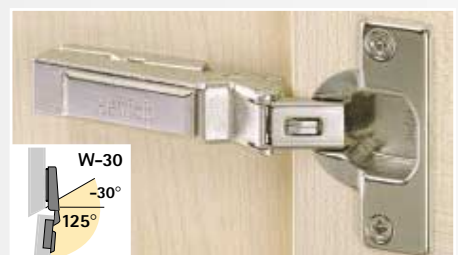
Intermat 9944 W-30 / 9944 W-30 FIX for negative cabinet angle -30° Opening angle 125° Pages 3.72 – 3.75
