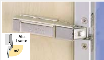
Intermat 9936 Alu for alu frame doors, opening angle 95° Pages 3.94 – 3.95 Sets Alu-frame doors Pages 3.96 – 3.97 Alu-frame profiles Pages 3.98 – 3.99
