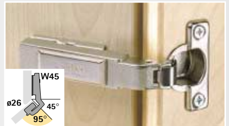
Intermat 9924 W45 for smaller doors/narrow frame doors Cabinet face angle 45° Opening angle 95° Pages 3.90 – 3.91
