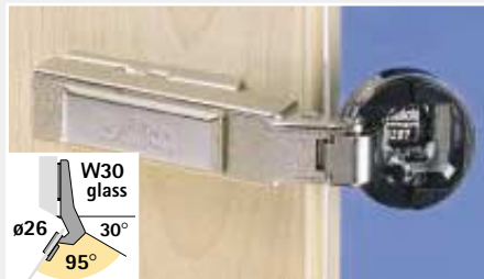
Intermat 9904 W30 for glass doors with cabinet angle 30° Opening angle 95° Pages 3.88 – 3.89
