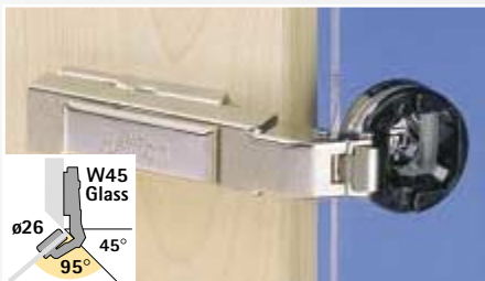
Intermat 9904 W45 for glass doors with cabinet angle 45° Opening angle 95° Pages 3.92 – 3.93
