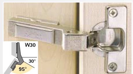
Intermat 9936 W30 / 9936 W30 FIX for cabinet face angle 30° Opening angle 95° Pages 3.58 – 3.61
